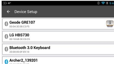
When you open the *Connect Device* screen, the Bluetooth devices available to your computer are displayed. If a Geode receiver is visible, it will be at the top of the list. If this is the first time you have paired with your Geode receiver, you may be asked for the pairing code, which is 0000.
