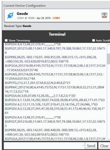
The lower end of the screen is a terminal window. This allows you to send queries and commands to the Geode receiver.
