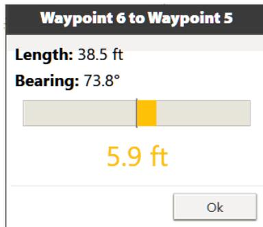
The centerline of the graph shows you the most direct path between waypoints. Deviations from that path are called *cross track errors*, and are shown as a shaded area to the left or right of the center line. The amount of error is also given, here shown as 5.9 feet.
