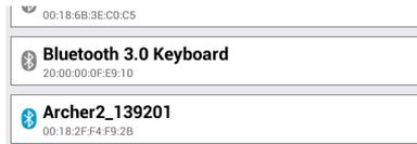
When you open the *Connect Device* screen, the Bluetooth devices available to your device are displayed. If a Geode receiver is paired, it will be at the top of the list. If this is the first time you have paired with your Geode receiver, you may be asked for the pairing code, which is 0000.
