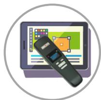
RPT100 is versatile UHF RFID & Barcode companion reader working with any existing Bluetooth enabled host devices such as a PC, smartphone or tablet running on OS Support of above Android 4.4, iOS7 and higher, Windows 10,8,7, Vista, XP, Mobile, CE, MAC. The RPT100 provides an economical and strategic way of extension to UHF RFID & Barcode reading.
