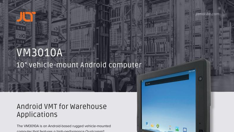
The VM3010A is an Android-based rugged vehicle-mounted computer that features a high-performance Qualcomm® Snapdragon™ 660 Octa-core CPU. The computer showcases enterprise mobility in a vehicle-mount computer form factor thanks to its rich I/O ports and versatile wireless connectivity options. The unit provides extra flexibility with the design of the dock including a one-click top latch that allows for easy
