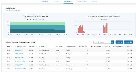
Real time analytics, powered by B2M Solutions, showing the health and performance of your estate of mobile devices, focussing on areas such as battery life, data usage, disruptions and connectivity. Enables the user to recognise patterns of usage and potentially pre-empt issues before they arise.
