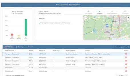
An additional “Smart” module that monitors device usage in more detail. Dashboard access provides information such as device location; user experience, including drop detection on Android devices and also enables alerts and geofences to be set up.
