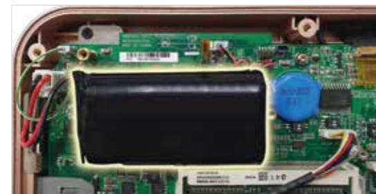
Back-up battery provides uninterrupted power
