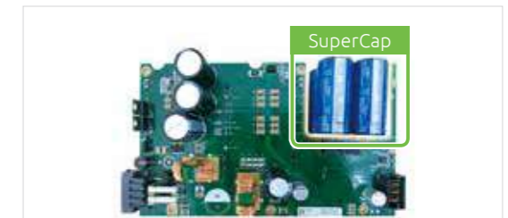
Protection for voltage dips
